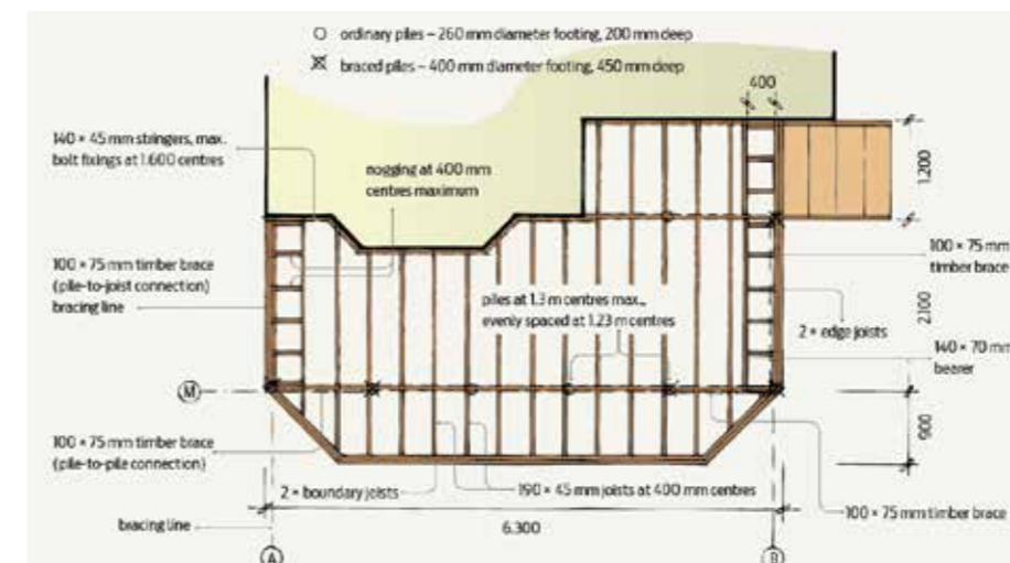
Figure 2: Proposed subfloor framing for the deck
