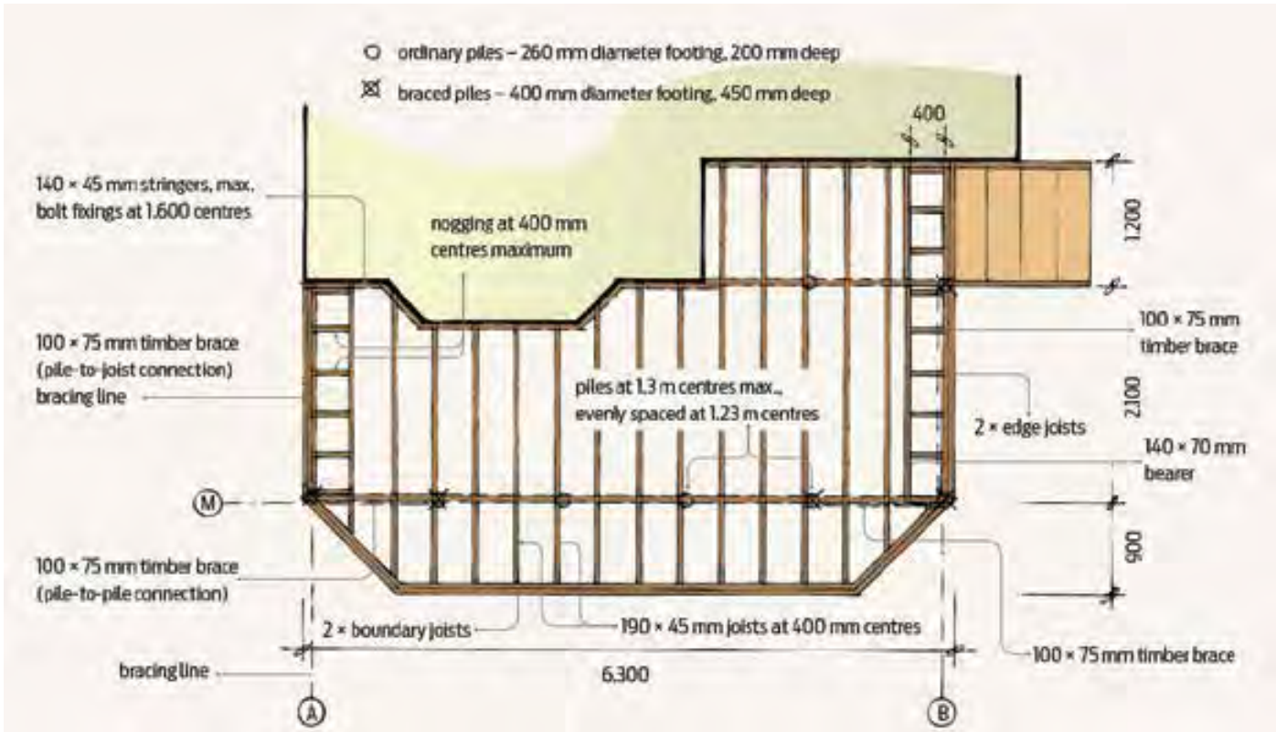
Figure 2: Proposed subfloor framing for the deck
